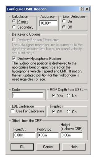
The *Accuracy* is the critical setting. This is generally between 7-15m, depending upon the performance of the USBL system. The lower the value, the greater the influence of the USBL data in the Kalman Filter. The higher the value, the less the influence of the USBL data in the Kalman Filter.
